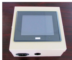
Remote Idec Touchscreen Control Panel
