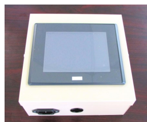
Remote Idec Touchscreen control Panel
